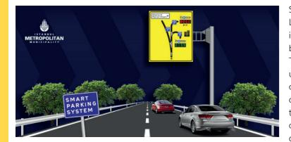
Smart Parking System is a LED-based dynamic parking lot information system developed by IMM's Department of Transportation. This system is used to provide real-time occupancy information of the closest parking lots to drivers on the roads. Parking lots' live occupancy information is displayed on LED screens and shown to drivers and it's updated 24/7 using live data transferred.
