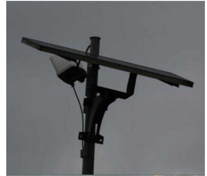
Traffic Sensor Powered by Solar Energy
